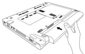
(Sample Illustration) Inserting the battery
